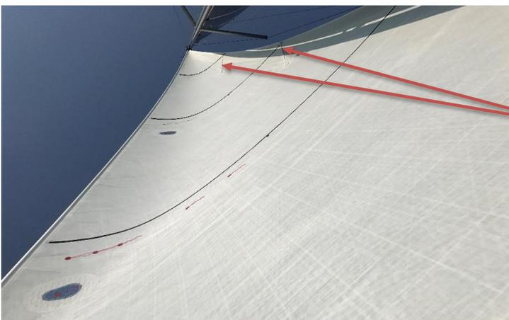
This is a 3Di Ocean 330 RF non overlapping jib with Vertical Battens to increase area. Note the fuller design shape to improve light wind performance.
