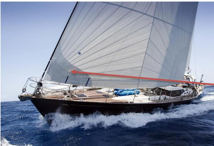
Roller Reef tack patch structure. Note the horizontally extended tack patch with reef position indicators along the foot for repeatable reefing amounts & to assist with matching the reefed clew position to a car setting marked on deck to match the new furled size.
